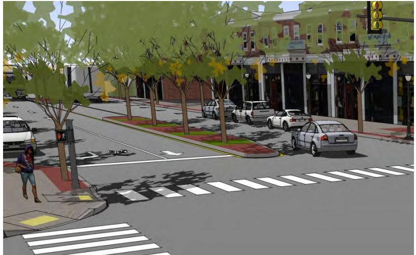
The above rendering – looking south (west) along Route 1 from Corbin Drive – illustrates the recommendations at this location including: curb extensions, landscaped curbed median, pedestrian crossing upgrades, and on-street parking.
