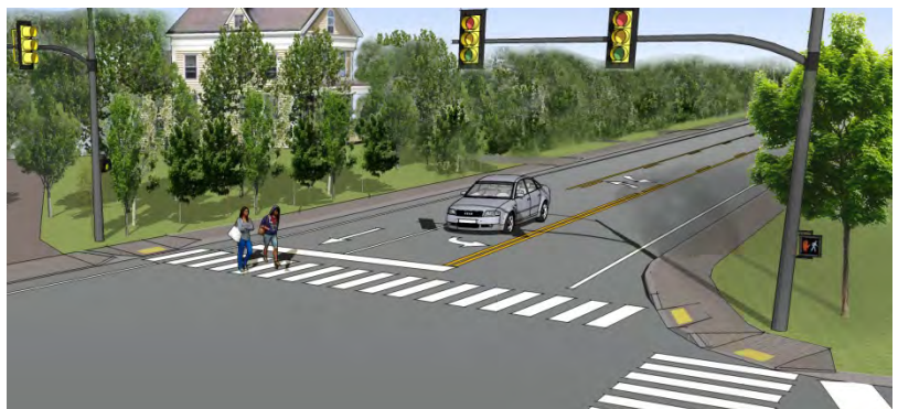
Looking north (east) along Route 1 from Old Kings Highway South. This rendering illustrates recommendations for a road diet, new sidewalk, and pedestrian crossing upgrades.
