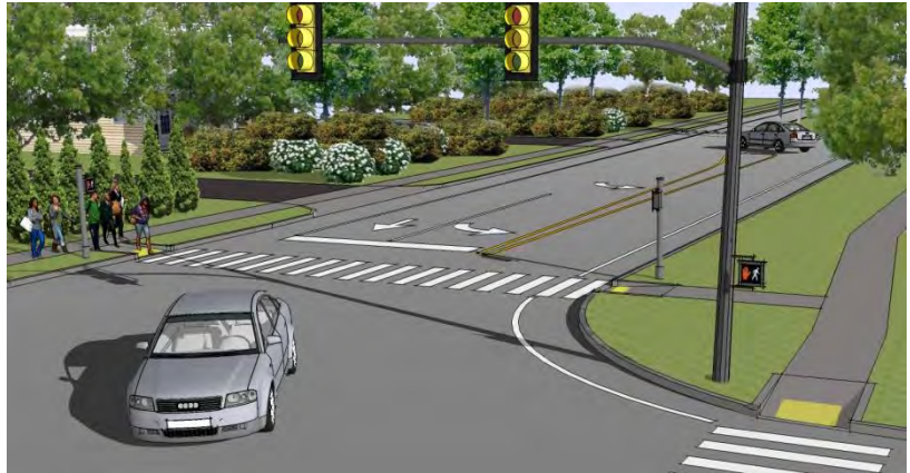
The above rendering – looking north (east) along Route 1 from Nearwater Lane – illustrates the recommendations at this location including: road diet, striped shoulders, corner radius reduction, and pedestrian crossing upgrades.
