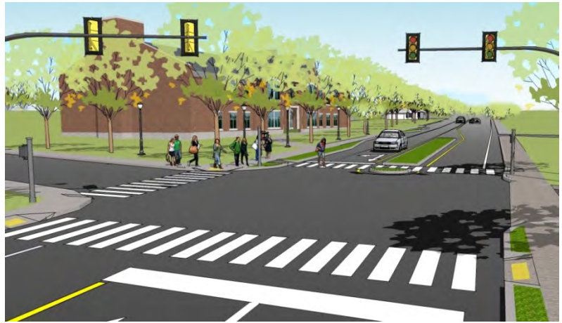
Looking north (east) along Route 1 from just south of Hecker Avenue. This rendering illustrates recommendations for a road diet, striped shoulders, curbed median, and pedestrian crossing upgrades.
