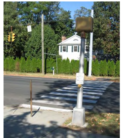
One of two pedestrian signals in the study area with exclusive crossing phases (that is, where no traffic moves concurrently with pedestrians) is located near the Hindley Elementary School at Nearwater Lane and Route 1.
