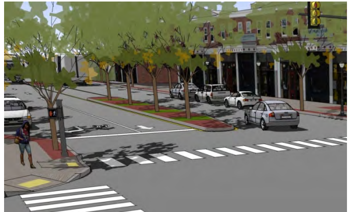
Looking south (west) along Route 1 from Corbin Drive. This rendering illustrates the recommendations at this location including: curb extensions, landscaped curbed median, pedestrian crossing upgrades, and on-street parking.
